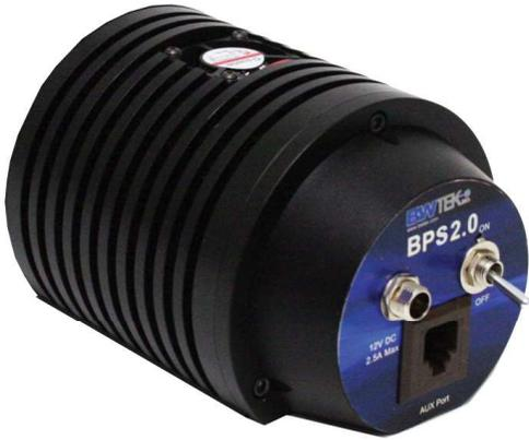
The BPS2.0 is a low-cost high-performance constant current light source which uses a replaceable Tungsten Halogen bulb rated for 2000 hours. This device uses a constant current setting which provides precision current control allowing for stable performance.
