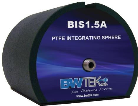
The BIS1.5 is a compact fiber coupled integration sphere. It is highly reflective (99% from 400nm-800nm) and Lambertian over the broad spectral range of 250nm-2500nm machined from PTFE.
